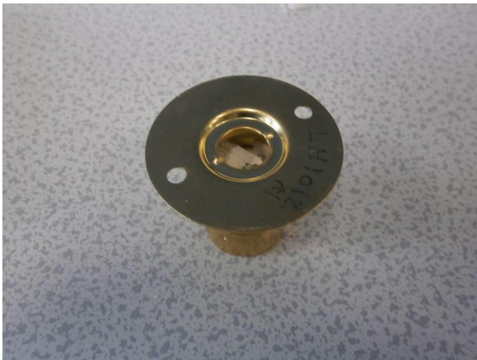
Illustration 4: Lampholder model 7707E assembled (view from cable entry)
